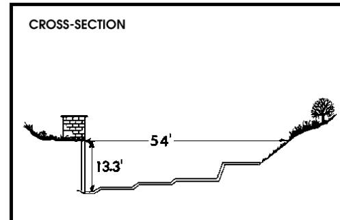
**RECORDER** - 5 min. interval data logger.**METHOD OF MEASUREMENT** - Wading**DRAINAGE AREA** - 6.36 square miles.**LOCATION** - 0.8 mile upstream of mouth of canyon and 3.0 miles northeast of Duarte.**REGULATION** - None.**DIVERSION** - None.**CHANNEL** - Natural, rock and gravel.**CONTROL** - Concrete control.**LENGTH OF RECORD** - July to September 1916; July 1917 to date.**REMARKS** - Operated and maintained by USGS until October 1, 1971.
