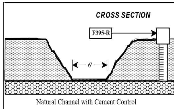
**RECORDER** - Continuous water stage.**METHOD OF MEASUREMENT** - Wading**DRAINAGE AREA** - 5.41 square miles.**LOCATION** - On left bank, 75 feet east of Mescal Canyon Motorway, 2.7 miles south of Fort Tejon Road, and 3.8 miles southwest of Pinon Hills.**REGULATION** - Slight regulation of low flow by Jackson Lake**DIVERSION** - One small diversion upstream from station for domestic use.**CHANNEL** -**CONTROL** -**LENGTH OF RECORD** - October 2001 to September 2005 discontinued.**REMARKS** -
