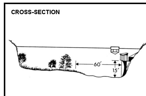
**RECORDER** - Continuous water stage.**METHOD OF MEASUREMENT** - Stream gaging.**DRAINAGE AREA** - 49.2 square miles.**LOCATION** - 2.0 miles above Little Rock Dam, 5.0 miles south of Little Rock.**REGULATION** - None.**DIVERSION** - None.**CHANNEL** - Sand, gravel, and boulder, natural in section.**CONTROL** - Channel forms control.**LENGTH OF RECORD** - October 1, 1930 to date.**REMARKS**
